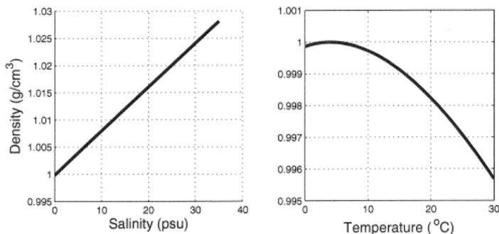
Figure 3.5. Density as a function of salinity and temperature.
