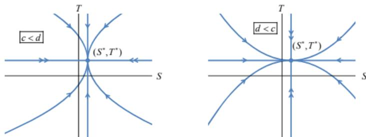
**Figure:** Phase portraits in the  $ST$ -plane. Solutions approach the sink tangent to the **slower** straight-line solution. Source: Dick McGehee, Univ. of Minnesota and MCRN, lecture slides.
