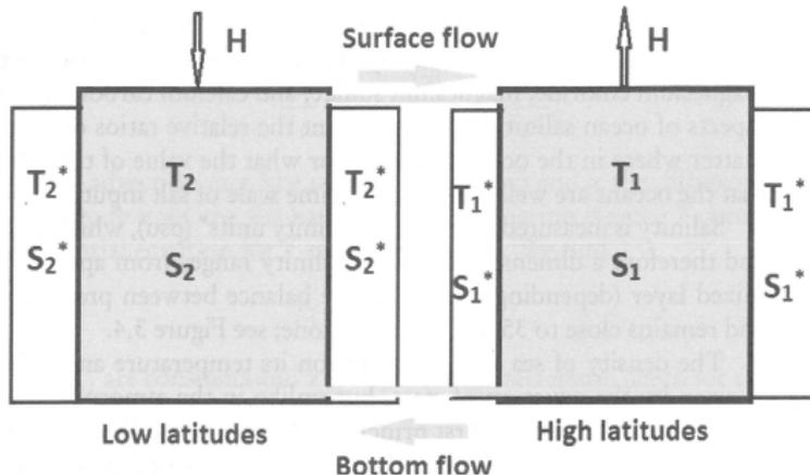
**Figure:** The two-box ocean model for temperature and salinity proposed by Henry Stommel in his paper “Thermohaline Convection with Two Stable Regimes,” *Tellus* **XII** (1961), 224–230. Source: Kaper and Engler, p. 34.
