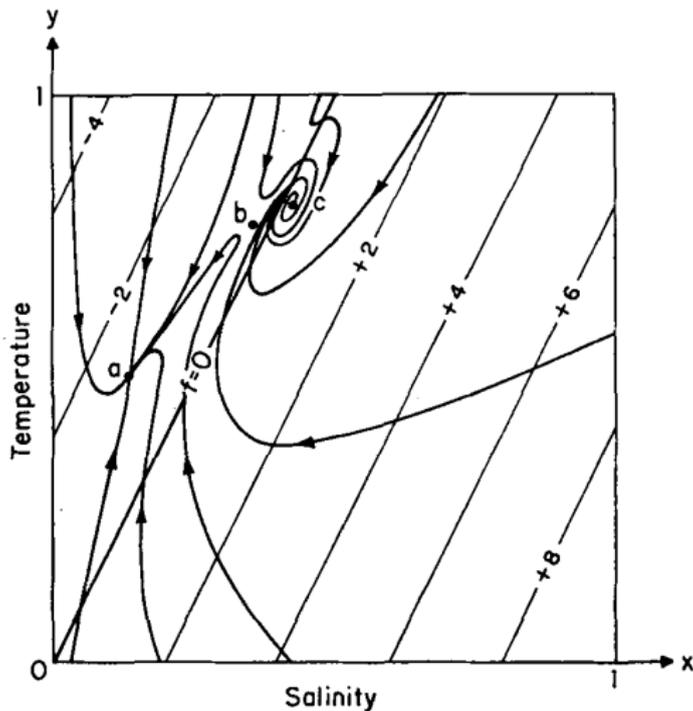
**Figure:** The phase plane for Stommel's reduced two-box model for parameter values  $R = 2$ ,  $\delta = 1/6$ , and  $\lambda = 1/5$ . There are three equilibria: **a** is a sink, **b** is a saddle, and **c** is a spiral sink. Source: "Thermohaline Convection with Two Stable Regimes," H. Stommel, *Tellus* **XII** (1961), 224–230.
