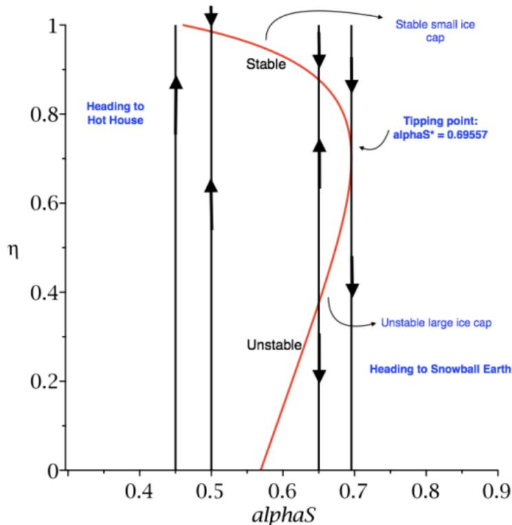
**Figure:** Bifurcation diagram showing the location of the ice line equilibria (roots of  $h(\eta) - T_c$ ) as the albedo parameter  $\alpha_S$  is varied. Note the saddle node bifurcation (tipping point) at  $\alpha_S \approx 0.69557$ . Figure by Cara Donovan.
