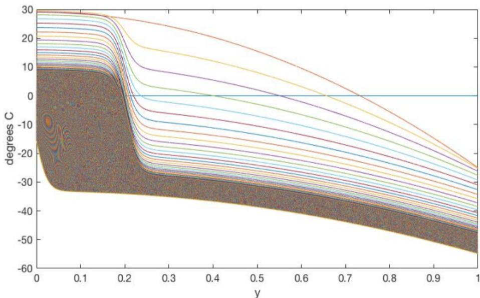
**Figure:** Iterations of the coupled Budyko-Widiasih model under Neoproterozoic conditions with  $\epsilon = 10^{-5}$ ,  $\eta_0 = 0.2$ ,  $\alpha_S = 0.65$ , and  $A(\eta) = \frac{220}{7}\eta + \frac{1216}{7}$ . Simulation took 7653 iterations to reach Snowball state ( $\eta = 0$ ). Figure created by Cara Donovan using Matlab.
