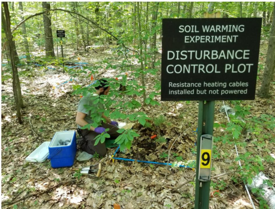
**Figure:** Soil Warming Experiment at **Harvard Forest**. Cables are buried in different plots to heat (or not) the soil  $5^{\circ}\text{C}$  above the ambient temperature in order to determine the effect on soil  $\text{CO}_2$  emissions. Figure Source: <http://harvardforest.fas.harvard.edu/photos/soil-warming-control-plot>
